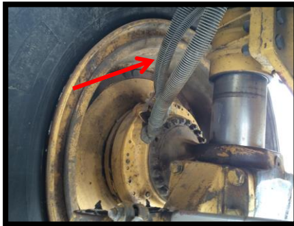
777D with Oil Cooled Front Brakes Remove hose & cap with #8 ORFS Install "Front Service Brake Tooling"
