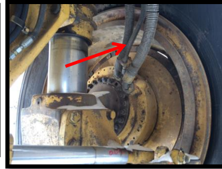
777D with Oil Cooled Front Brakes Remove hose & cap with #8 ORFS Install "Front Service Brake Tooling"
