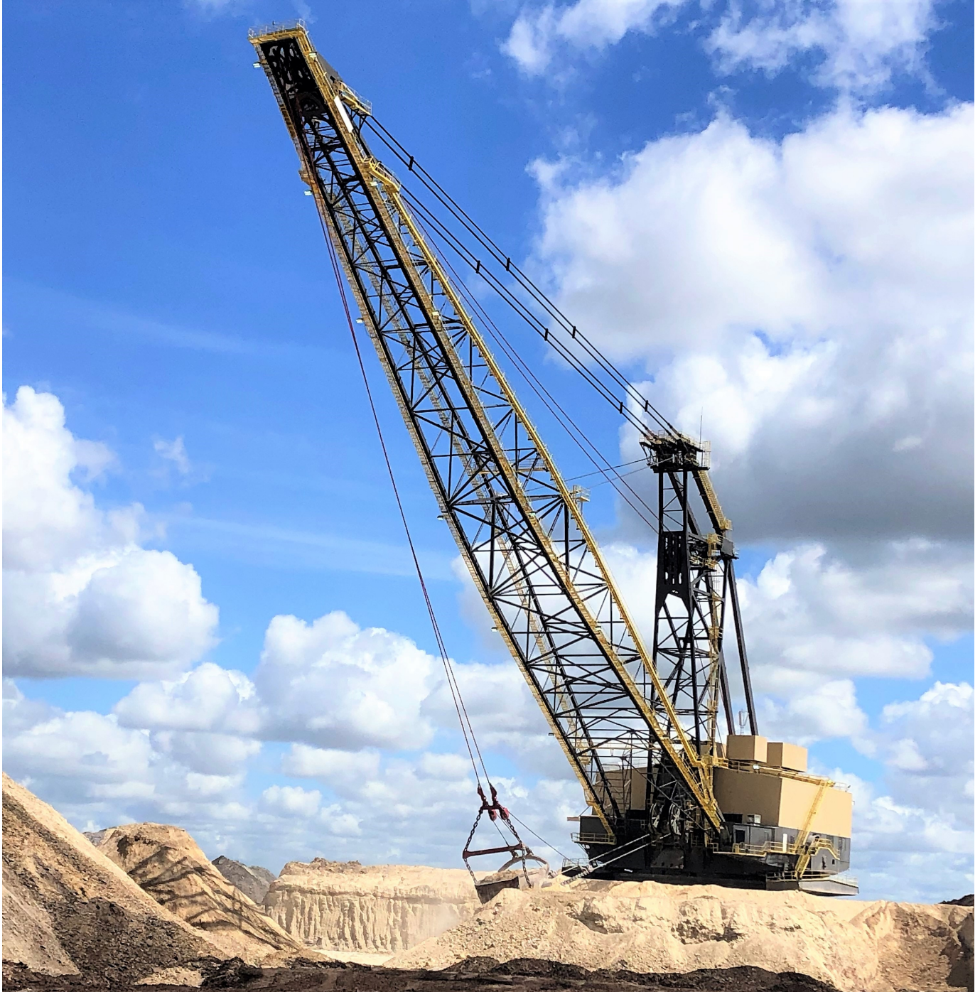
Picture taken July 2020, Marion 8200 dragline in operation at thermal coal mine in San Miguel, Texas
