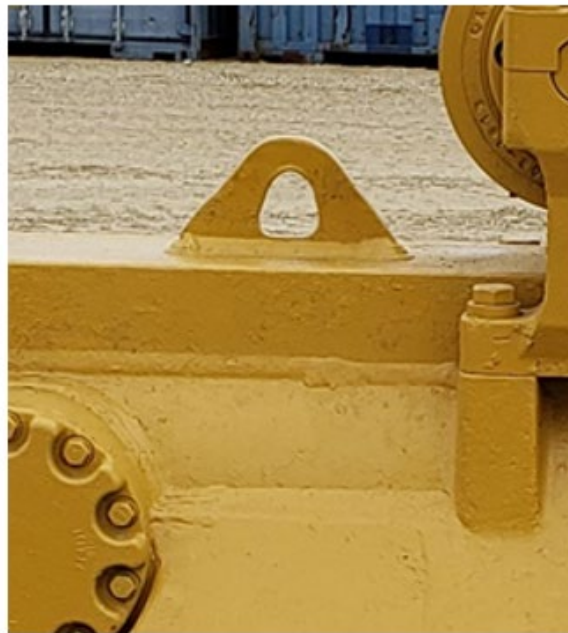
Example of a good lifting lug.
