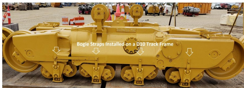
Bogie straps installed on a D10 track frame.
