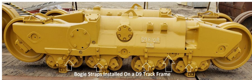
Bogie straps installed on a D9 track frame.
