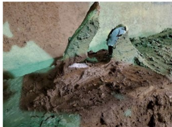
Example of a lifting lug failing during lifting operations.
