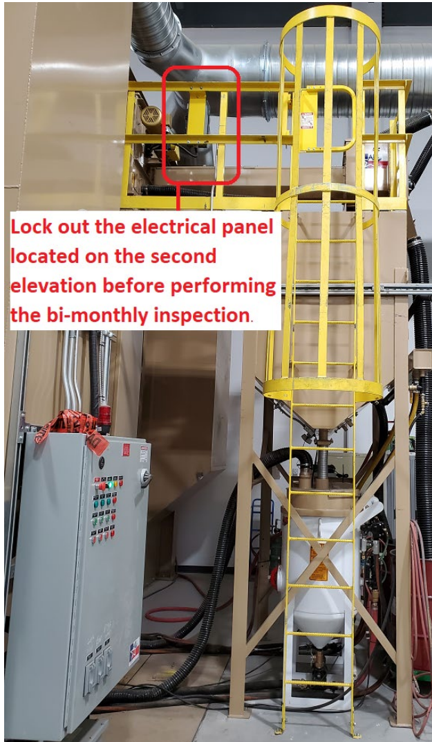
ABS – Below Floor Sweep in Recovery Blast Room
