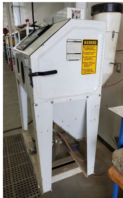
Mod-U-Blast Cabinet Abrasive blaster – Used for small parts and components
